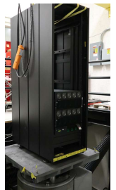
Operational S&V with the workload running un- interrupted
