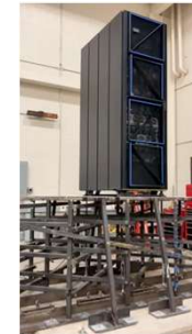
Earthquake simulating Richter 8.3 scale with the workload running un-interrupted
