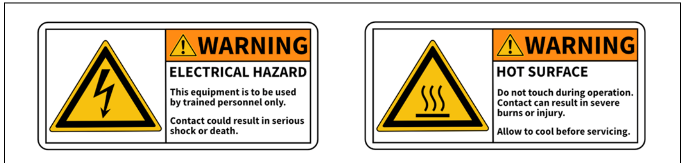
Figure 2 Electrical hazard and hot surface warnings
